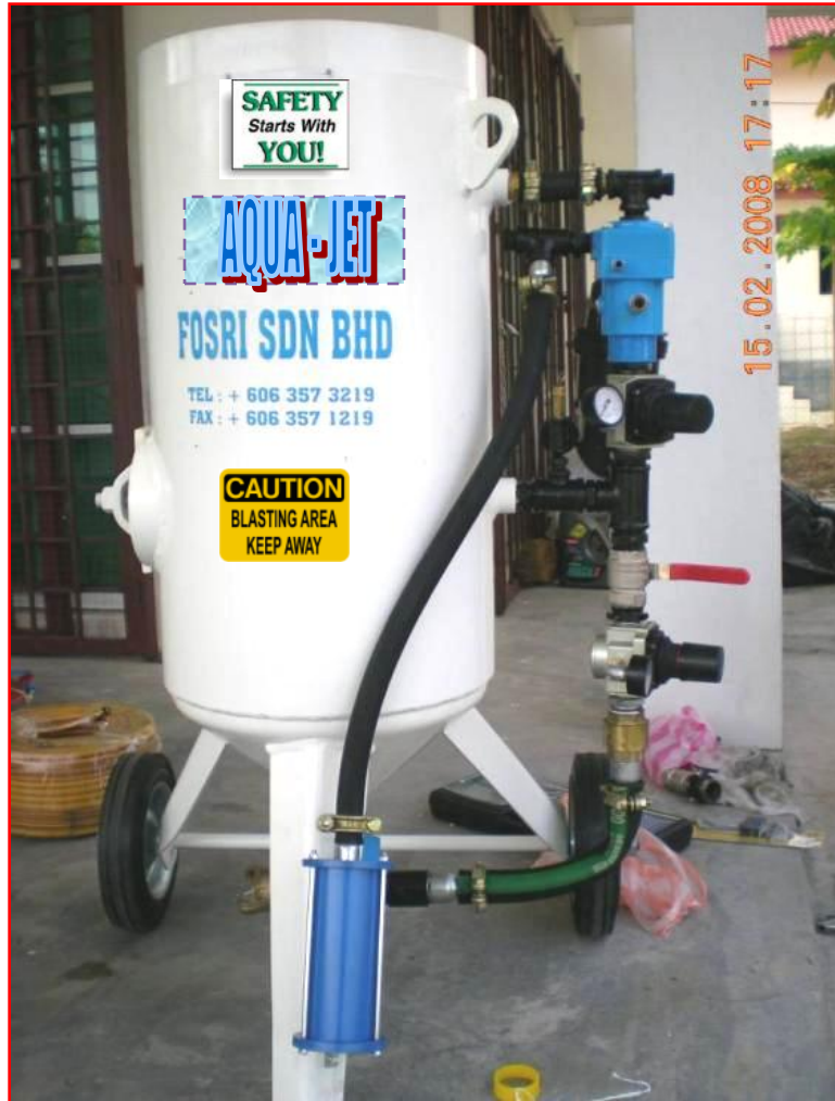
The Wet Abrasive Blast System with controlled pressure, water and media capabilities
